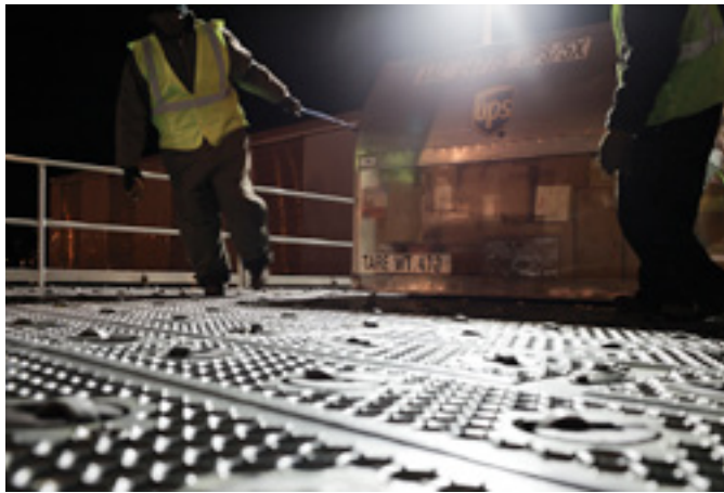
“Ballmat” roller platforms allow workers to glide air containers weighing several thousand pounds into and out of UPS aircraft
